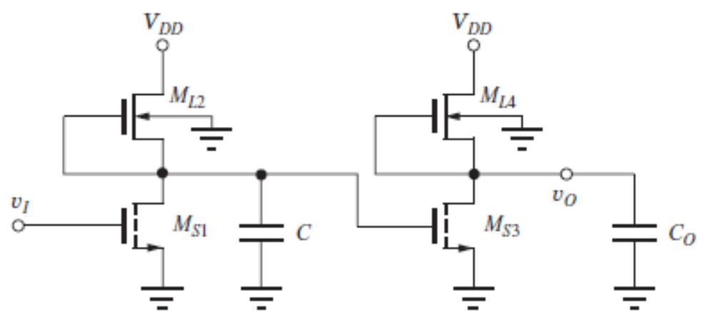
The capacitances on a given node can be lumped into a fixed effective nodal capacitance  $C$
